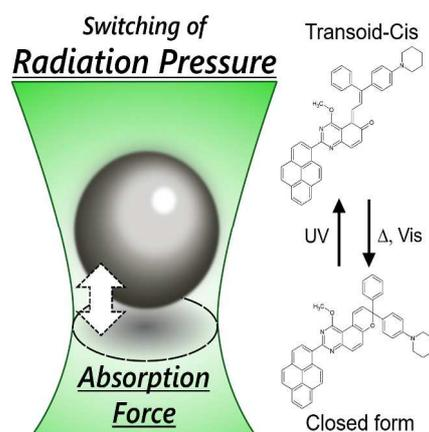
**Figure 1.** Schematic illustration of switching of radiation force by using photochromic reactions of NPs.
