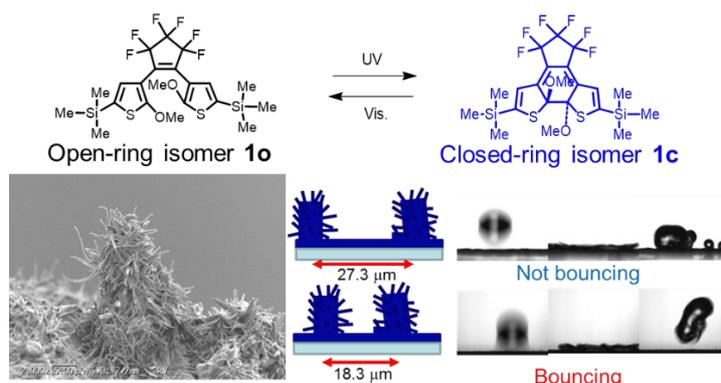
**Figure 1.** Molecular structure of **1**, and side view SEM image of diarylethene double roughness structure, and water drop bouncing phenomena on two different surfaces with different intervals between the larger size projections. Scale bar: 5  $\mu\text{m}$ .
